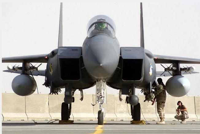
*USAF F-15E equipped with LANTIRN pods (the rounded attachments in front of the wheels).<sup>6</sup>*
