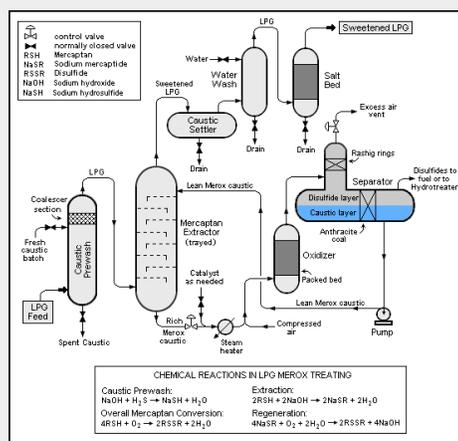
*A process flow diagram devised by a chemical engineer describing the Merox process for removing mercaptans from liquid petroleum gas.<sup>2</sup>*
